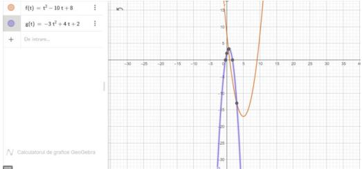
The vehicles meet twice, because the second vehicle stops. 2.2 Uniform Rectilinear Motion
